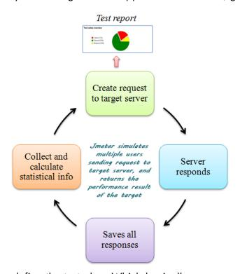
To use JMeter, one need to define the test plan. Which basically means, one must specify
